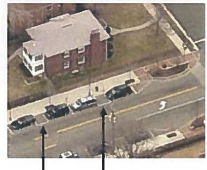
Maneuvering zones in between shorter on-street spaces guide cars to leave larger gaps to ease entering and exiting on-street spaces.
